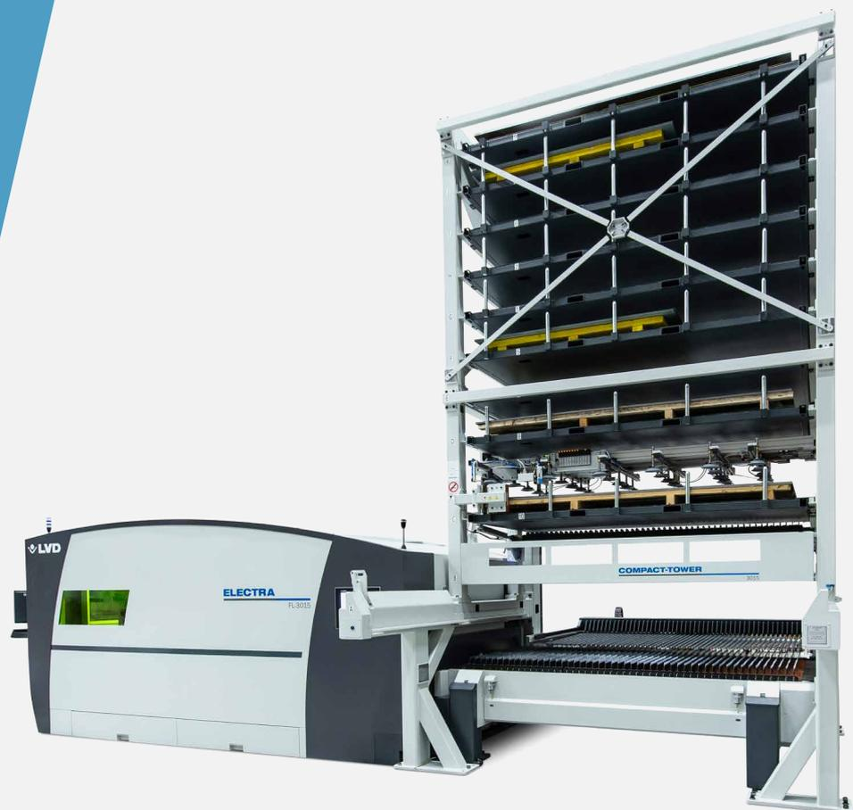
The Compact Tower for Lasers (CT-L) 3015 is a cost-effective tower for loading, unloading and storage of raw materials and finished parts. It is offered in four configurations: 4, 6, 8 or 10 pallets. The system handles 3050 x 1525 mm sheets and material thicknesses up to 25 mm with a pallet storage capacity of 3000 kg. The CT-L unit facilitates unmanned production in a compact environment.
